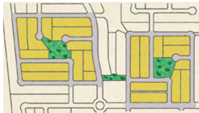
Fig. 1 - Part of a larger subdivision plan, two neighbourhoods show the guideline spirit: loops and cul-de-sacs form a complete walking network by means of parks. They also become "places" centered on open space.
