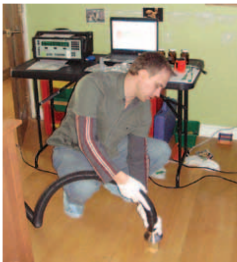
Dust collected in a specialized vacuum is analyzed for semi-volatile organic and biological compounds related to the presence of mould and bacteria.
