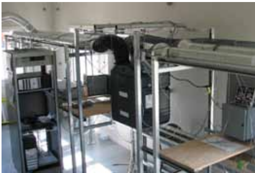
Figure 1: Testing of an HRV/ERV system in a specially designed test rig
