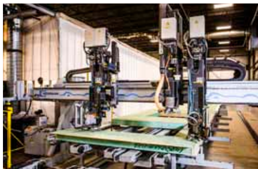
A wall panel has sheathing secured in place with computer numerically controlled (CNC) machines.
